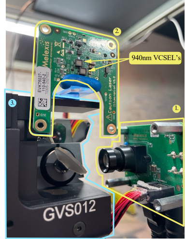
a. Hardware setup with Melexis ToF camera with one row ROI and scanning with Galvos
